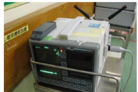
Active RFID tag affixed onto a medical device for its location tracking
