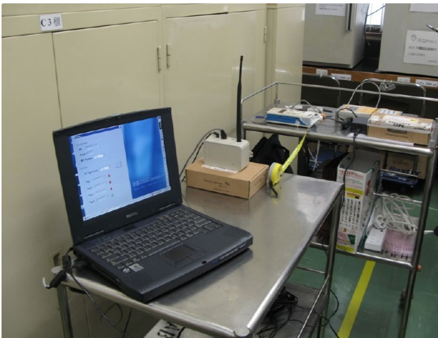
EMI Assurance Test Setup
