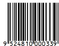
Figure 4.14-5. Example of EAN-13 with EAN/UPC HRI format
