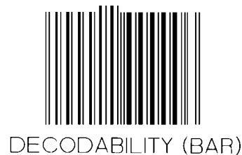
Figure 5.12.5.12-3. Calibration symbol with engineered low decodability grade
