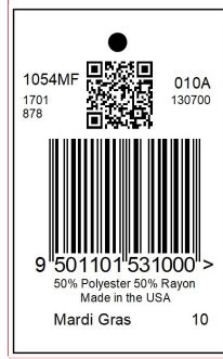
Figure 6.3.3.1-4. Maximum POS X-dimension 2D barcode placement in relation to the linear barcode example
