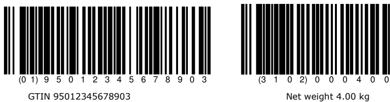
Figure 5.10.2.1-1. Data encoded in two GS1-128 symbols
