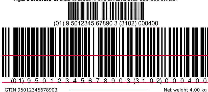
Figure 5.10.2.1-2. Data encoded in one concatenated GS1-128 symbol
