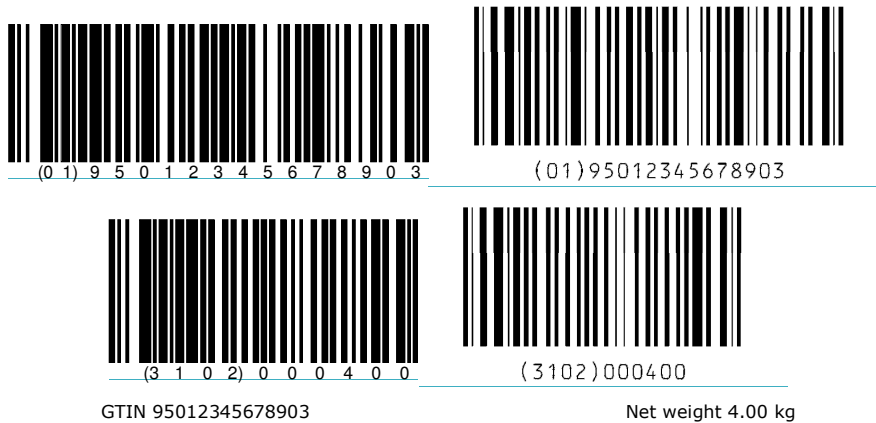
Figure 5.10.2.1-1. Data encoded in two GS1-128 symbols
