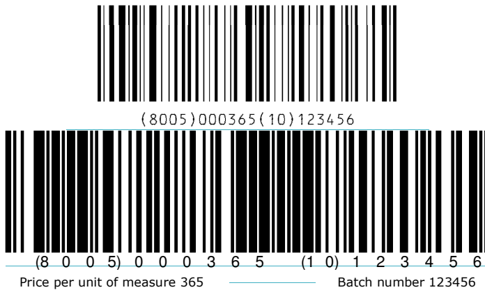
Figure 5.10.2.2-2. Data encoded in one concatenated GS1-128 symbol
