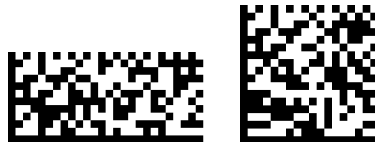
Figure 5.7.3.1-1. Rectangular and square GS1 DataMatrix symbols (Specific applications are not used in the data encodation. Both symbols contain the same data)
