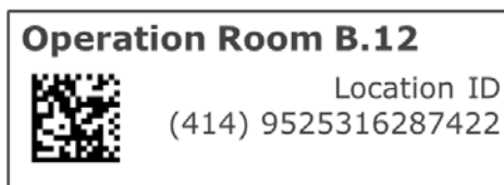
Figure 4-1 Application Identifier (414) – GLN of a physical location
