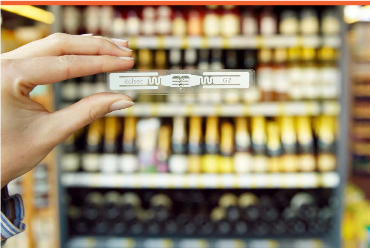
To be effective, it is necessary to control the management of tags at the time of assigning the GTIN for each bottle since the omission and duplication of tags can cause inventory differences of the products shipped. One of the lessons learned: Metal containers affected tag reading since the metal acts as a barrier.
