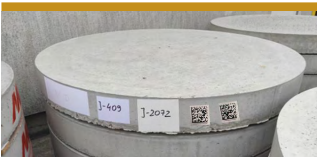
Fig. 2. Example of 2D GS1 DataMatrix code
