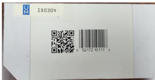
Figure 4-13 Co-located barcode with QR Code (GS1 Digital Link URI) leading the UPC-A
