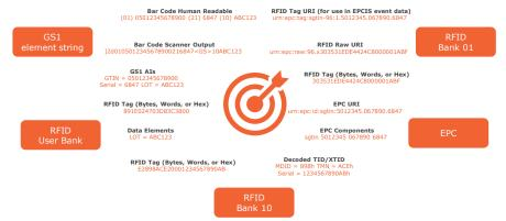
For example, these classes allow you to easily translate data from the output of a barcode scanner directly into bitstream encoded into the EPC memory of an RFID tag. You can also easily encode multiple AIs into the User memory bank using the Packed Object compaction method and much much more...
