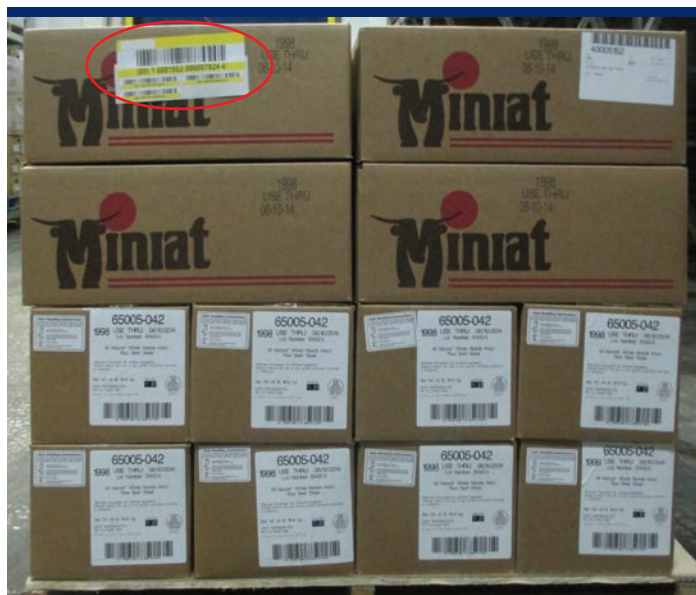
Supplier cases are linked to a GS1 Serial Shipping Container Code (SSCC) encoded in a GS1-128 barcode on a hybrid pallet label for ease of delivery receipt at Chipotle’s distribution centers.
