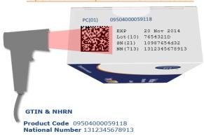
The product code line is part of the artwork rather than printed on line. Printing 5 lines of text at a readable point size adds technical constraints on the production lines.
