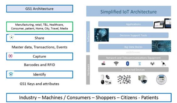
The foundation layer to IoT is the Connected Devices. These devices include barcode, RFID readers and sensors that act as interfaces between uniquely identified objects and the next layers of the architecture where data are transferred, stored and analysed. The triggers are on the one hand the machines executing tasks in an industrial IoT context and on the other hand human beings seeking experiences or efficient ways to do things.
