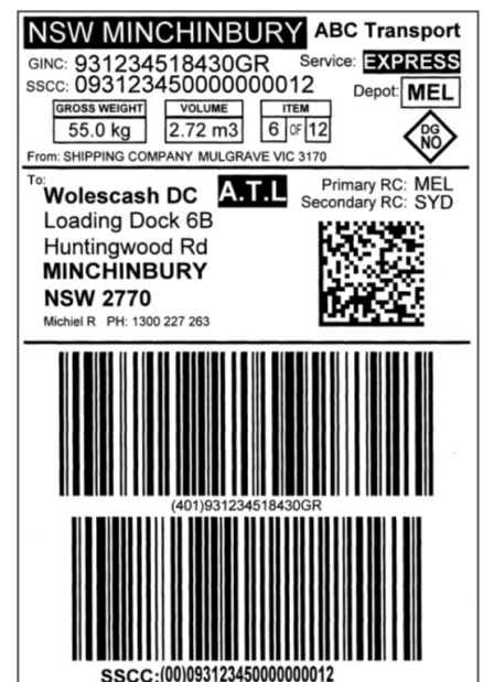
Transport label with 2D barcode (Data Embedded barcode)
