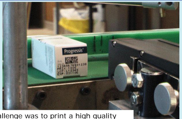
The challenge was to print a high quality grade Datamatrix code (orthogonal) and 4 lines of text at a time on a moving carton without decreasing the speed (35m/mn) and on an area not exceeding 30x20mm (carton flap)
