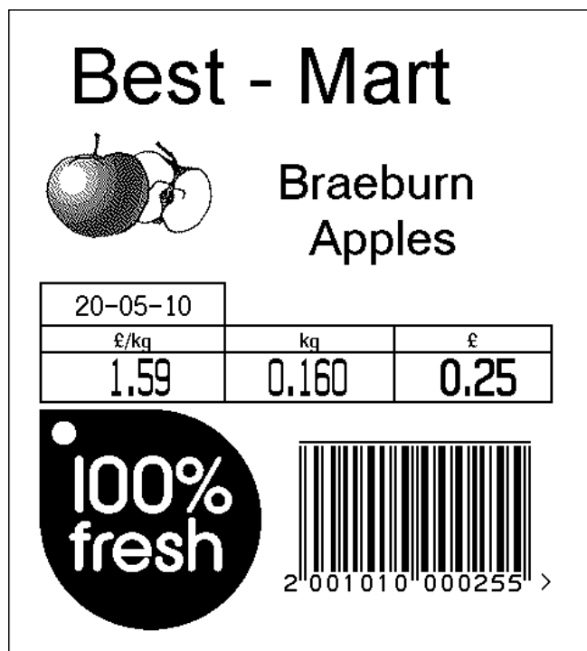
Figure 5-1: Current label using EAN-13 encoding an RCN with a Prefix 02 / 20-29
